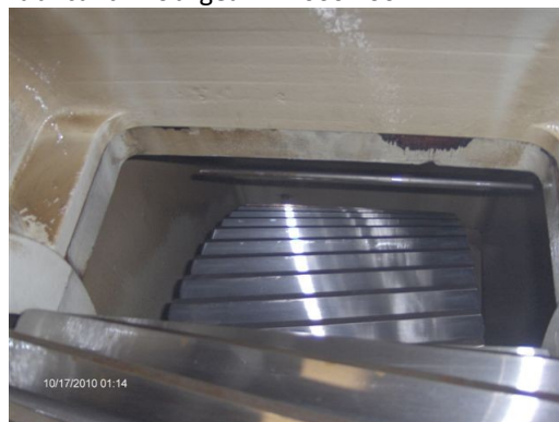
Scana Volda, 2000Kva, 1800 Kw, Lubricant: Mobilgear XP 600 100
